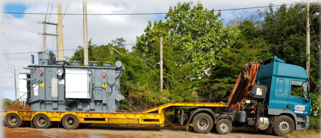
Transportation and Fixing of 22/66KV TX
